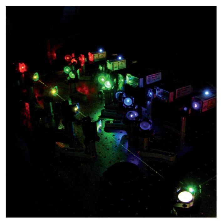
With the help of different mirrors, red, green and blue laser beams are layered over one another before being bundled into a single beam within the fluorescent microscope. They are used to make previously marked proteins fluoresce. This method enables researchers to examine individual elements and the structure of a cell.
